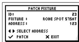
The address can also be shown as binary. It is shown direct below the decimal address on the left side of the display. Further it's possible to create fixture libraries, such as moving lights, scanners etc. Up to 32 different fixtures with up to 35 channels each can be manually entered in the XMT-120A. When these fixtures are patched, you will always see the description of the actual channel on the bottom of the
